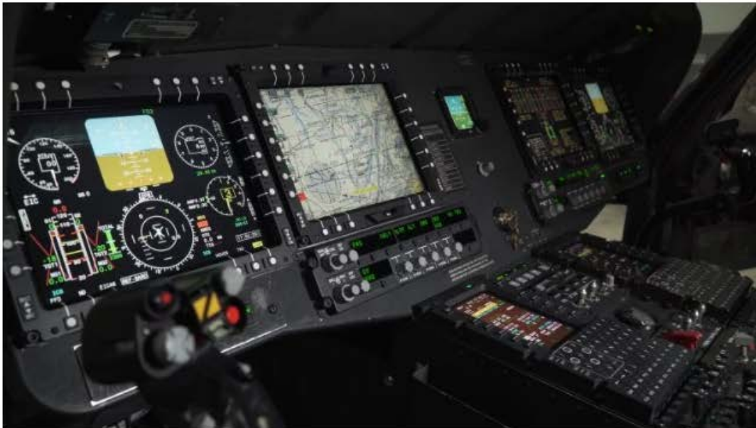
The digital, open-architecture cockpit of the upgraded UH-60V "Victor" Black Hawk
